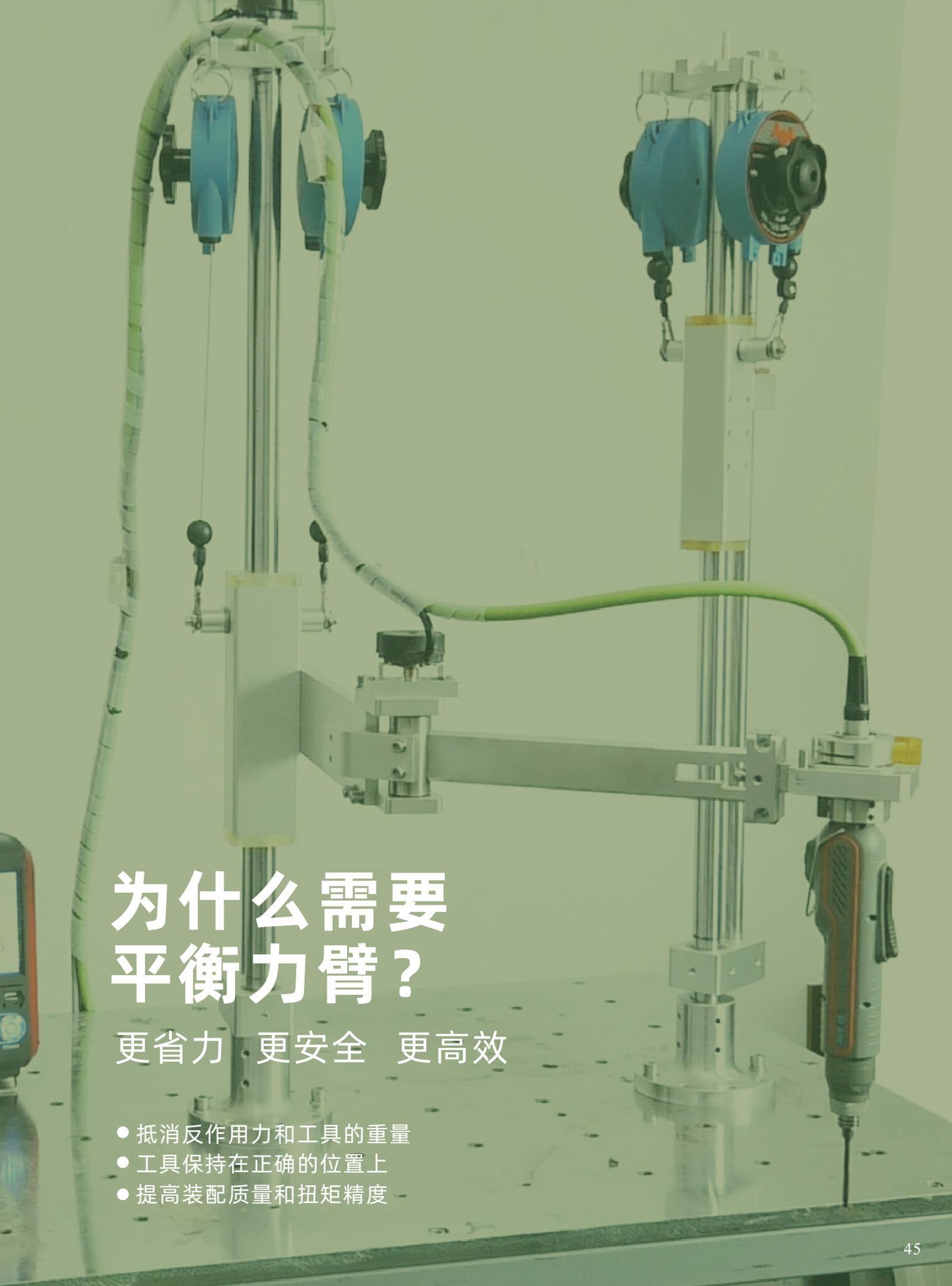
The image shows a mechanical assembly station. It features a vertical column with a horizontal arm extending from it. A power tool, possibly a screwdriver or drill, is mounted at the end of the arm. The tool has a grey handle with orange accents and a black shaft. The arm is supported by a complex mechanism of pulleys and cables, designed to balance the weight of the tool. The background is a plain, light-colored wall.
